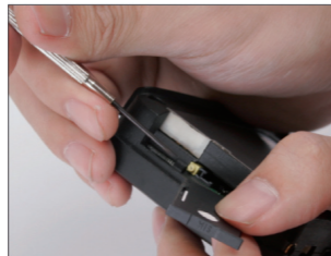
Removing the SIM holder.
